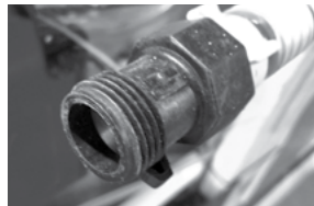
Unscrew the cap off of the connector, then screw your garden hose to the threads of the connector
